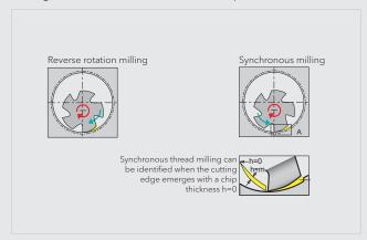
For thread milling, synchronous milling should be applied whenever possible, in order to achieve lower cutting forces, improved chip formation, longer tool life and better surface quality.
