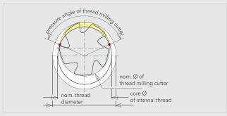
The diameter of the thread milling cutter and the profile depth determine the pressure angle to the thread diameter.
